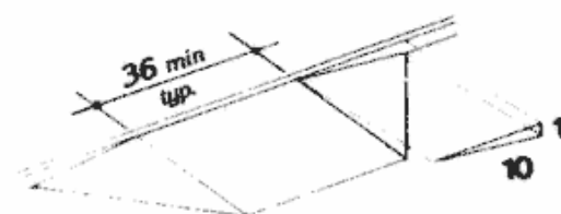
Fig. 13 Built-Up Curb Ramp
